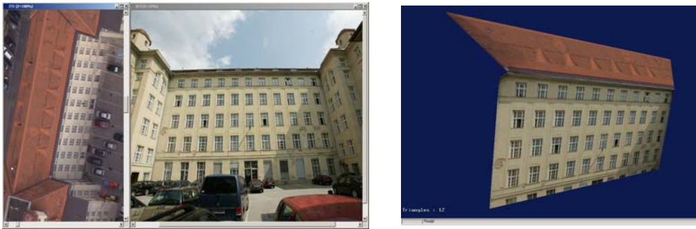
Figure 7: Three-dimensional model of a building (right), obtained from aerial photography (left) and augmented with terrestrial photography (center).
